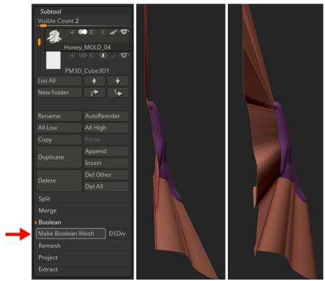
9. Using boolean unions and differences, build out any necessary functional mold parts such as a base, sprues, and keys.
