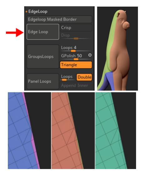
5. Expand the edge of the first part (I usually start with the biggest), working in sections to avoid inversions and undercuts in the parting plane.
