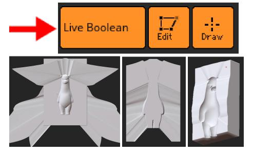
8. Repeat these steps with the other parts, but push the edge loops forward across the parting plane as you expand them out so that each can be booleaned away by the preceding parts. This will ensure a good fit with no gaps.
