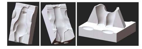
10. **Decimate** the parts if necessary in the **Zplugin > Decimation Master** pallet, and export the parts as .**STL** files in the **Zplugin > 3D Print Hub** pallet.
