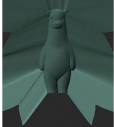
For interior facing edges, expand towards the midline until they meet, then **Weld Points** in **Geometry > Modify Topology** pallet
